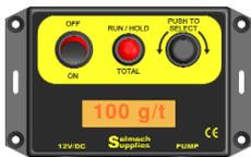
Enter the application rate of your additive in litres per tonne.
